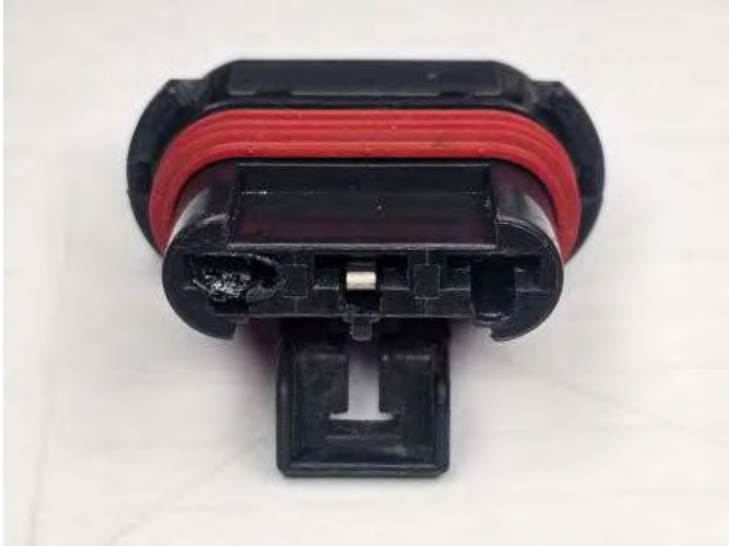
Front of melted plug. Metal connector in left slot still there but covered by melted plastic.
