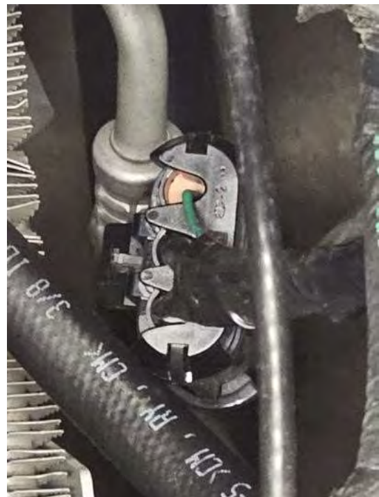
Close up of plug showing smaller green wire that was reused
