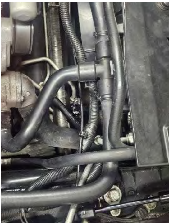
Location of plug, behind right side of radiator.
